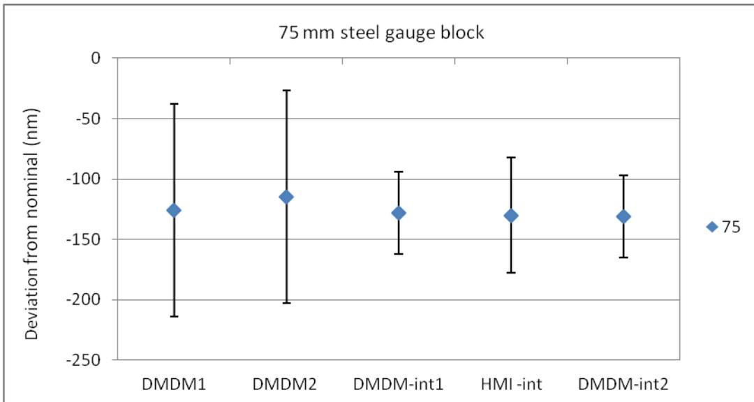
**Figure 2(d)** Deviation in Central Length of 75 mm gauge block
