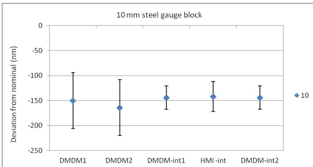
**Figure 2(b)** Deviation in Central Length of 10 mm gauge block
