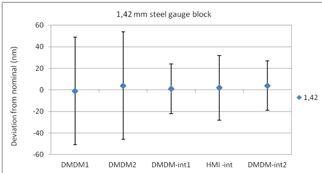
**Figure 2(a).** Deviation in Central Length of 1,42 mm gauge block
