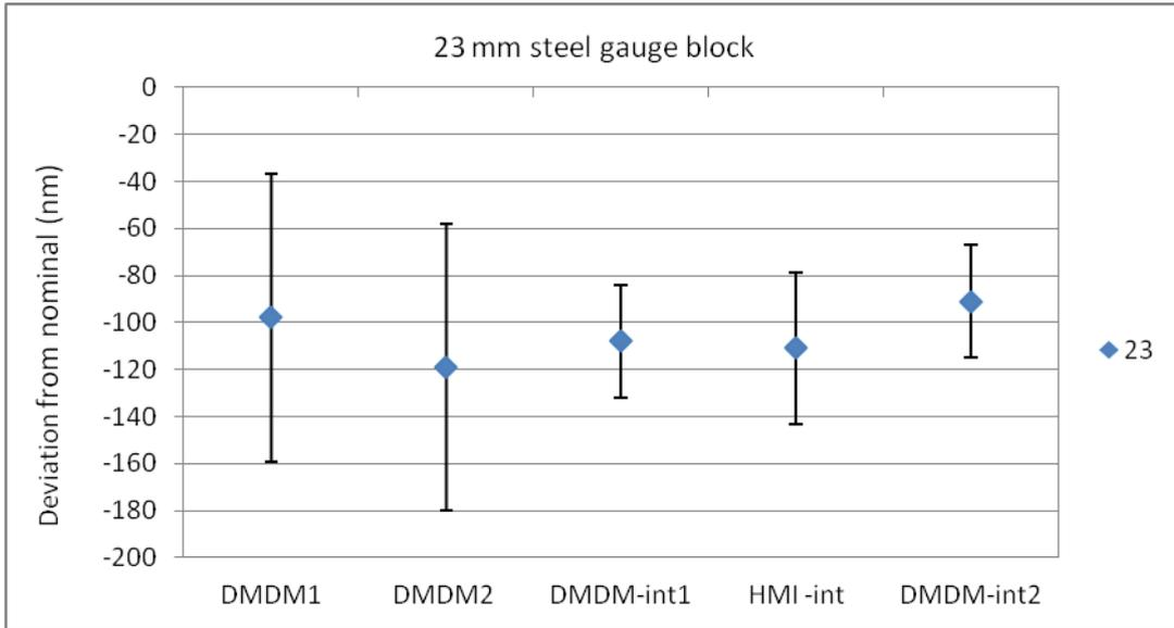
**Figure 2(c)** Deviation in Central Length of 23 mm gauge block
