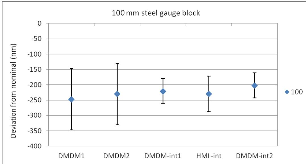
**Figure 2(e)** Deviation in Central Length of 100 mm gauge block
