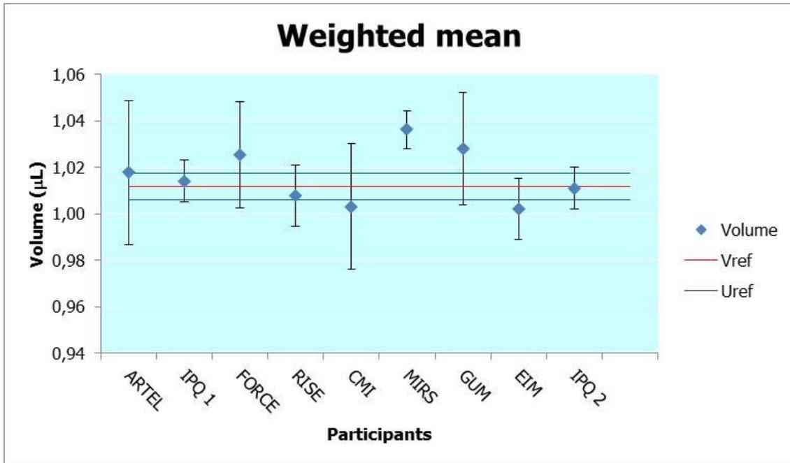
Figure 6 – Volume results with reference value – 1 µl
