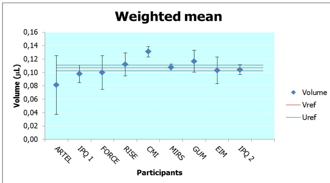
Figure 7 – Volume results with reference value – 0,1 µl
