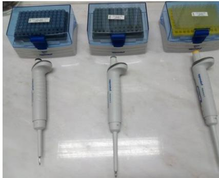
**Figure 1-** Fixed Micropipettes
