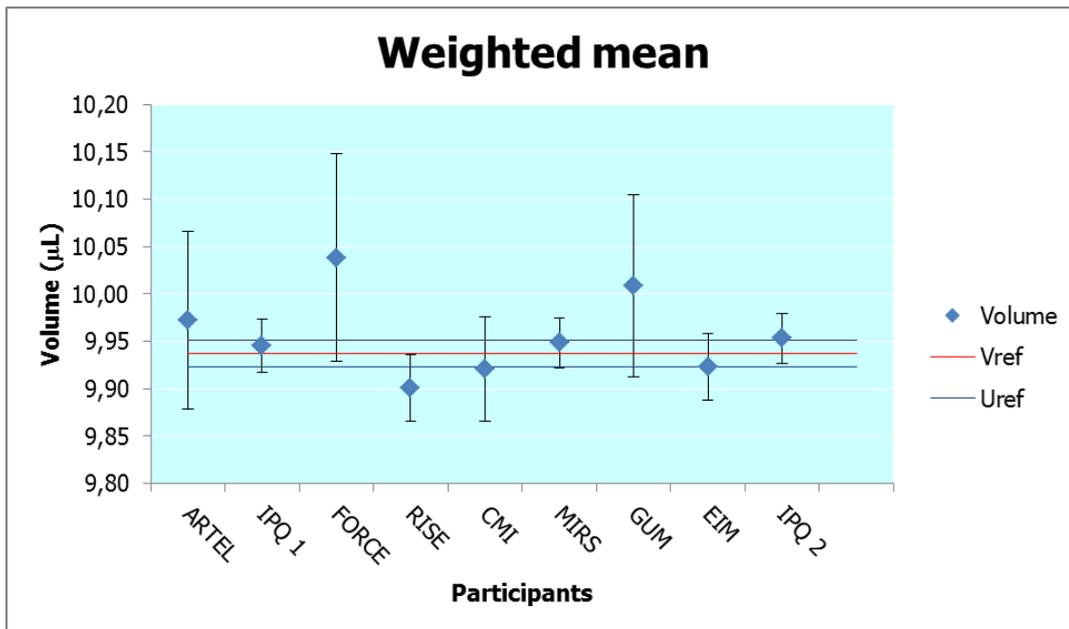
Figure 5 – Volume results with reference value – 10 µl
