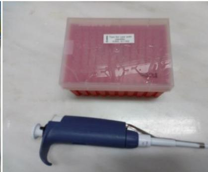
**Figure 2 -** Variable Micropipettes
