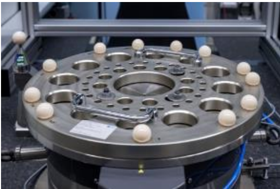
Figure 18: The new circular ball plate mounted on a rotary table. It can be seen that the spheres do not have uniform angular spacing.
