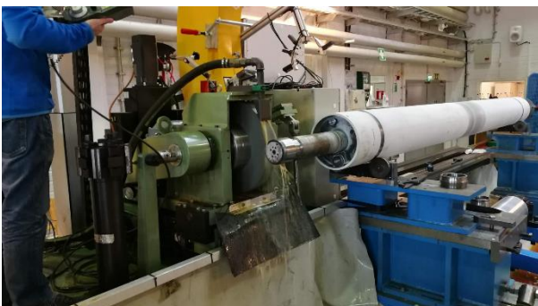
Figure 17: Compensative 3D grinding of the bearing installation tapered site. The tapered section was ground to the profile which minimised the roundness error of the assembled bearing inner ring raceways.
