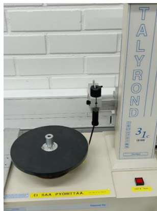
Figure 4: Left: Measurement of a reference workpiece using the developed ROMES three-probe roundness measurement device. Right: Measurement of a reference workpiece with a Talyrond roundness measurement instrument.
