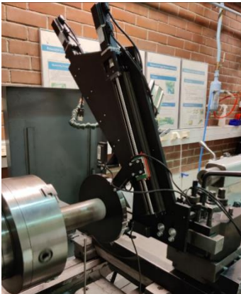
Figure 4: Left: Measurement of a reference workpiece using the developed ROMES three-probe roundness measurement device. Right: Measurement of a reference workpiece with a Talyrond roundness measurement instrument.
