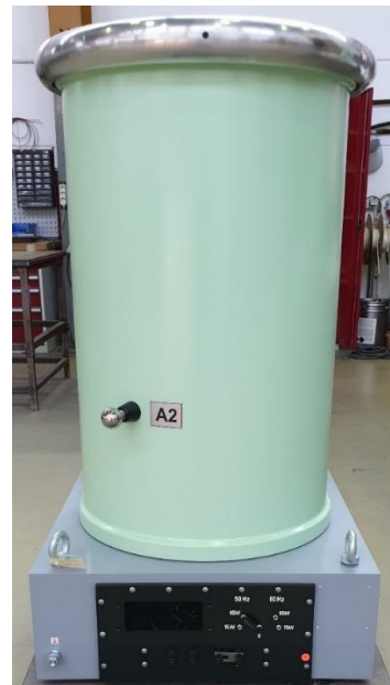
Figure 2. EPRO voltage channel based on 100 kV inductive voltage transformer.
