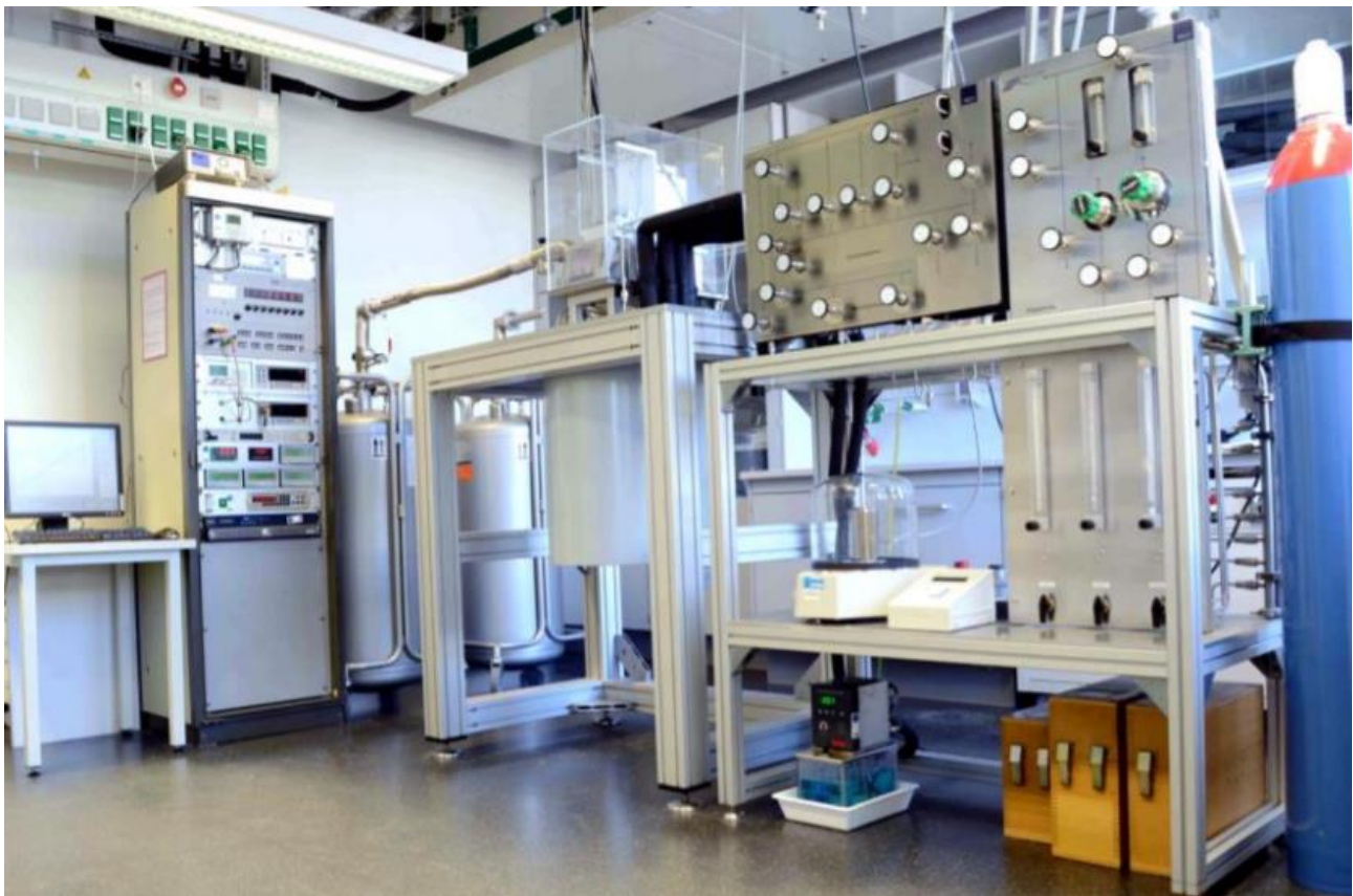
Figure 12: Photograph of the cryogenic densimeter set up at the thermodynamics institute of Ruhr University Bochum. Picture taken from [16].
