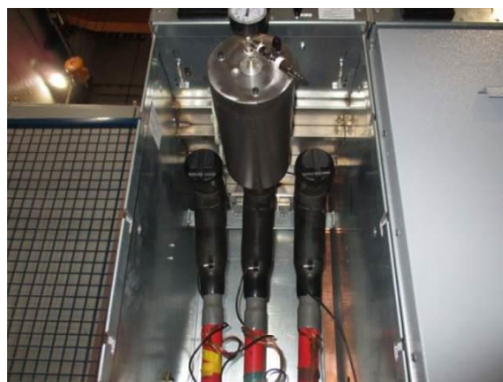
Figure 24: The voltage probe connected to medium voltage switchgear during ac test.
