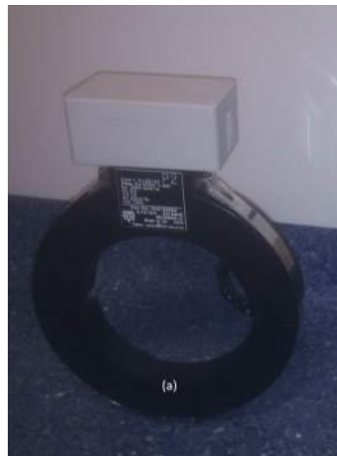
Figure 21: Transducers using fiber Bragg grating for readout. Left: 11 kV voltage transformer. Right: 1.2 kA split core current transformer
