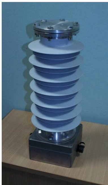
Figure 21: Transducers using fiber Bragg grating for readout. Left: 11 kV voltage transformer. Right: 1.2 kA split core current transformer
