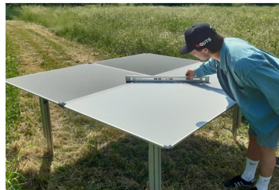
Figure 20: Reference reflectance panels being levelled in the field.
