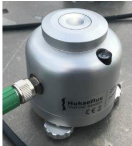
Figure 36: Spectrally flat pyrgeometer and its characteristics.
