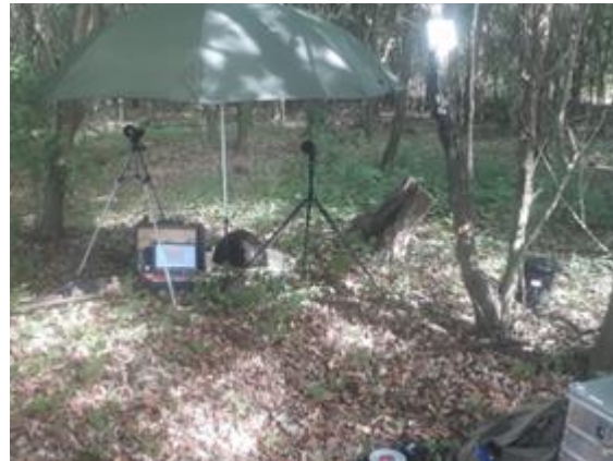
Figure 16: Figure of the setup for a measurement of sound pressure near a wind park, two microphones on tripods are seen under the umbrella, on the ground the microphone mounted on a board with additional extended wind screen.
