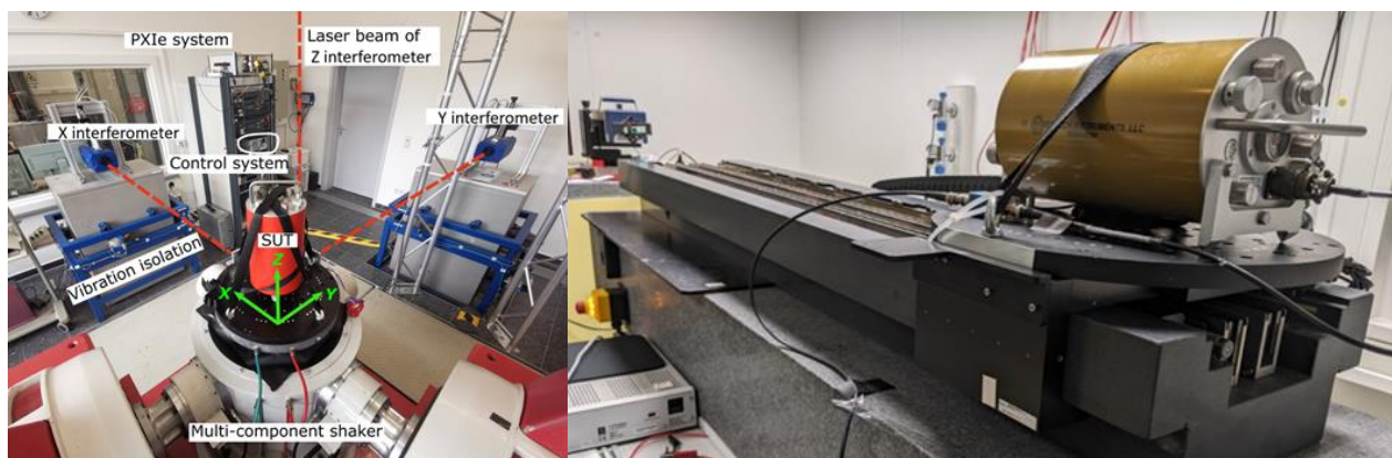
Figure 4: Primary calibration set-ups for the calibration of seismometers in three degrees of freedom at the multi-component exciter at PTB (left) and for horizontal calibration at the long stroke exciter at PTB (right).
