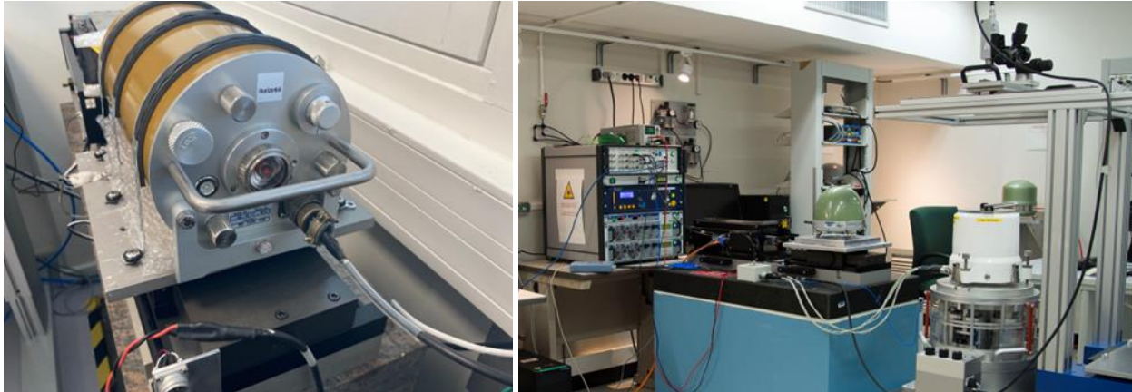
Figure 5: Primary calibration set-ups for the horizontal calibration of seismometers at HBK (left) and for horizontal and vertical excitation at CEA (right).
