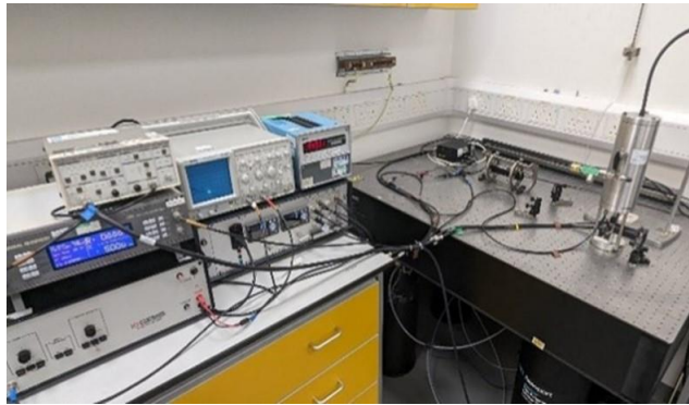
Figure 6 A photograph of the laser pistonphone set up at NPL and sensitivity level of a Brüel & Kjær (B&K) 8104 reference hydrophone.
