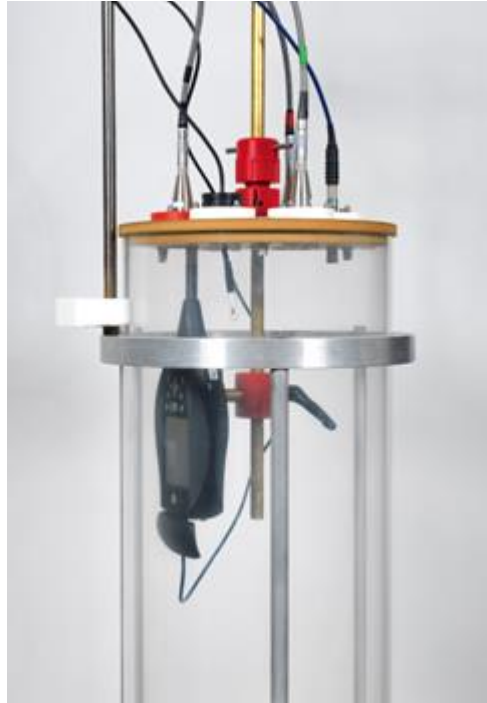
Figure 8: Devices under test mounted in the sound tube.
