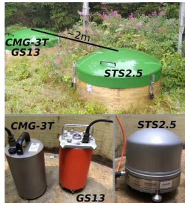
Figure 17: Seismometer models and their installation in the ground
