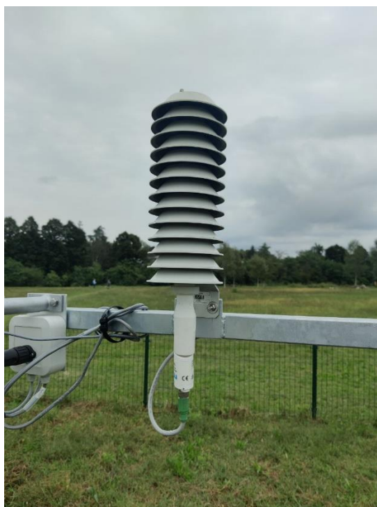
Temperature 2 (Naturally ventilated shield – thermohygrometer)
