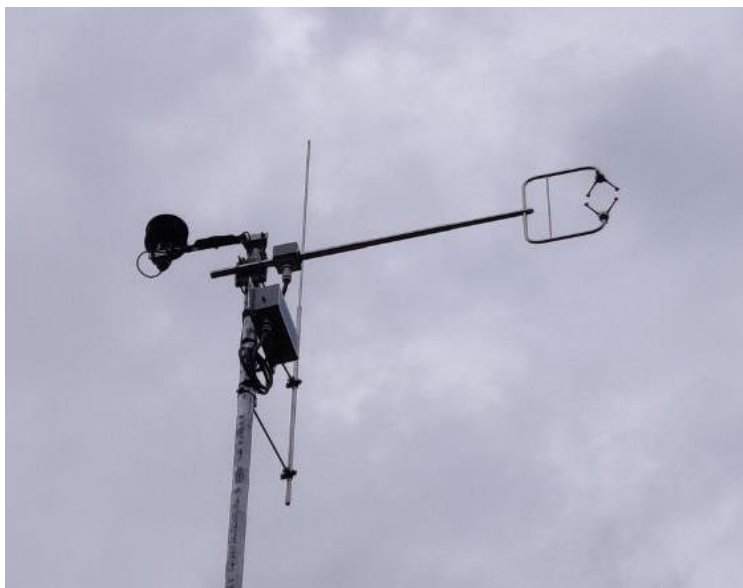
Wind Reference @10 m (GILL HS50 3 Axis)
