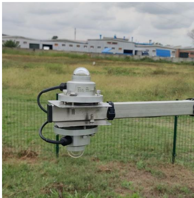
Direct and reflected radiation (2 Hukseflux pyranometers)
