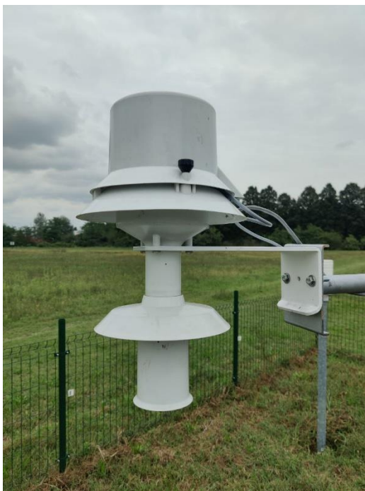
Temperature 1 (Artificially aspirated shield – PT 100)
