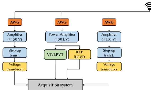
**Figure 13:** Schematic representation of the three phase generation and measurement system developed at INRIM for the characterisation of VT and LPVT under PQ disturbances and in presence of single and combined effects of adjacent phases and proximity effects.
