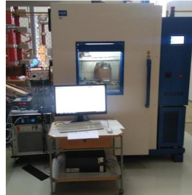
**Figure 11:** a) Schematic representation of DUT system for the characterisation of VT in presence of PQ disturbances under the single and combined effects of temperature and burden, b) picture of the DUT inside the climatic chamber.
