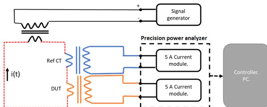
**Figure 7:** Schematic overview of the CT characterisation system. Generation of the high primary current, the CT-under-test (DUT) and the reference CT (which is, in fact, an electronically compensated current transformer), a precision power analyser, and the host computer.
