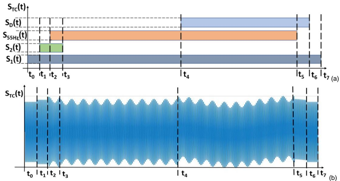
**Figure.1** Example of time combined waveform: a) time combined waveform scheme and b) time domain numerically simulated signal with  $h=2$ ,  $i=55$  Hz and subharmonic at 1 Hz.
