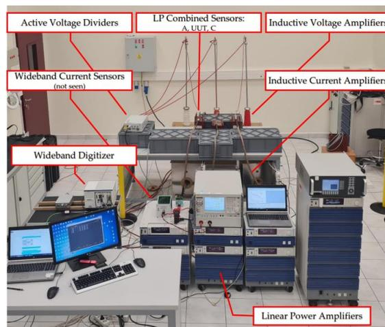
**Figure16 – TUBITAK three-phase measurement set-up for the characterisation of combined ITs and LPITs in presence of influence factors**
