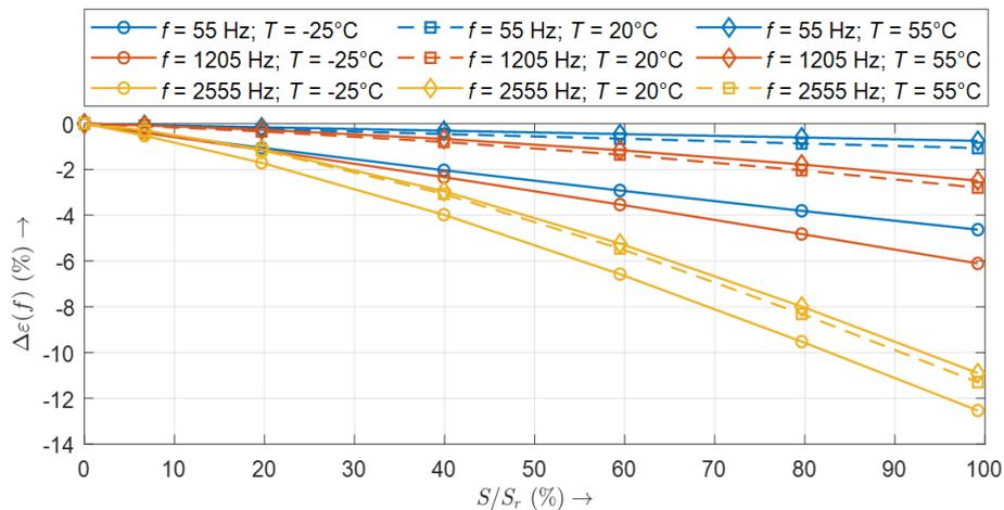
**Figure 12:** VT responses at three inharmonic frequencies (55 Hz, 1205 Hz and 2555 Hz) as function of burden measured under three different temperatures (-25 °C, 20 °C and 55 °C).
