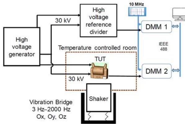
**Figure 9:** Schematic representation of the reference generation and measurement system for the characterisation of IT in presence of PQ disturbances under the single and combined effects of temperature and vibration
