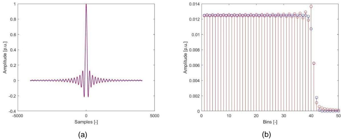
**Figure 8:** Time domain (a) and frequency domain (b) representation of the windowed sinc function (blue) and the basic one (red).
