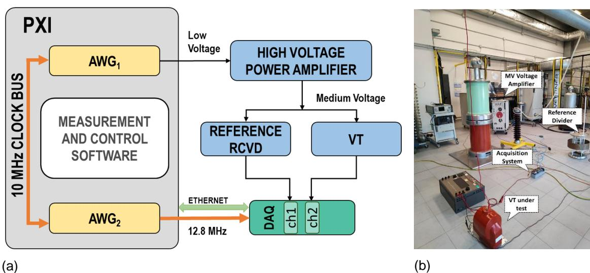
**Figure 2:** INRIM reference generation and measurement system for VT and LPVT characterisation in presence of PQ disturbances: (a) scheme and (b) laboratory set-up.
