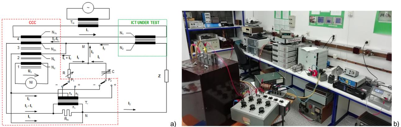
**Figure 4:** CMI alternative reference generation and measurement system for CT characterisation in presence of PQ disturbances, based on the use of a home developed CCC; a) scheme; b) laboratory reference set-up.
