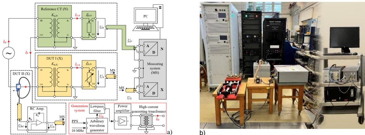
**Figure 3:** PTB reference generation and measurement system for CT and LPCT characterisation in presence of PQ disturbances: (a) scheme and (b) laboratory set-up.
