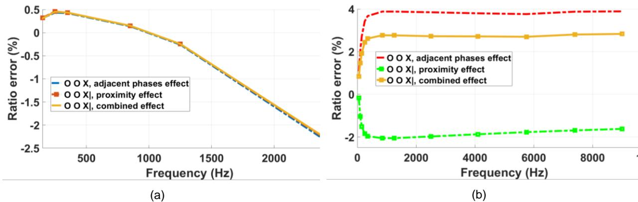
**Figure 14:** VT (a) and resistive-capacitive LPVT (b) frequency ratio error responses under single and combined effects of adjacent phases and proximity.
