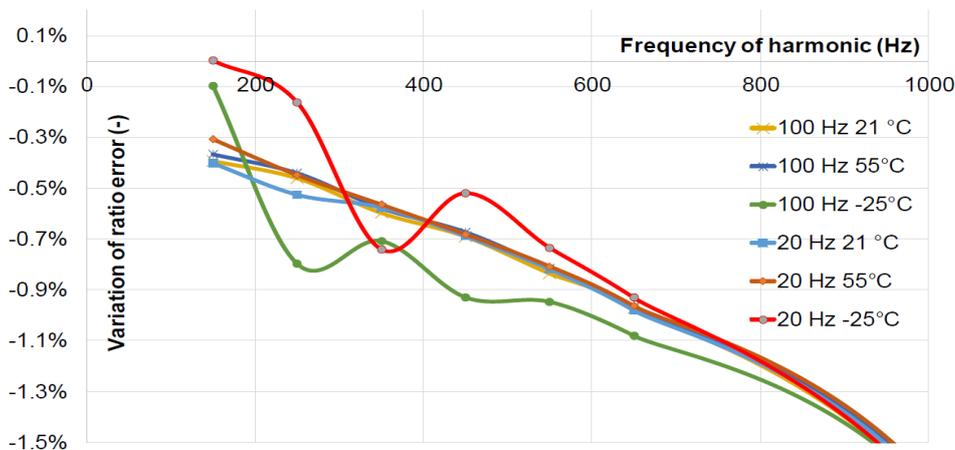
**Figure 10:** VT harmonic response up to 1000 Hz measured under bi-tone voltage test waveform in presence of different vibration frequency and temperatures.
