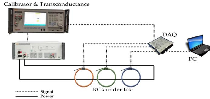
**Figure 15:** Schematic of the UNIBO measurement setup.
