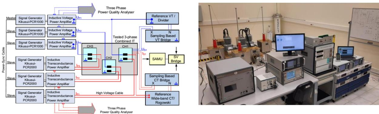
**Figure 5:** TUBITAK reference generation and measurement system for combined IT characterisation in presence of PQ disturbances: (a) scheme and (b) laboratory set-up.
