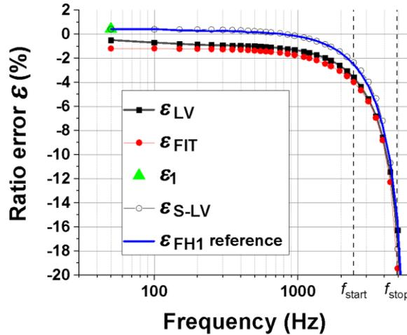
**Figure 6:** Representation of the SINDICOMP-LV steps for the identification of the VT ratio error frequency response compared with a reference MV frequency response.
