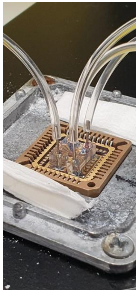
Figure 10: 12 channel GFET sensor with fluidic interface.
