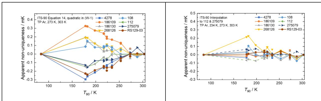
Figure 11: Type 3 non-uniqueness uncertainty without (LHS) and with (RHS) the mercury triple point included in the interpolation. Although the type 3 NU increases a little without the use of the Hg triple point the increase is still small
