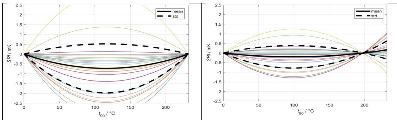
Figure 8. On the LHS the type 1 NU in the range Zn:Sn using the ITS-90 formalism and on the RHS the type 1 NU in the same range using the least squares approach
