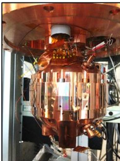
Figure 14: A photograph of the quasi-spherical acoustic resonator used by INRIM for the proof-of-concept implementation of improved primary thermometry using Refractive Index Gas Thermometry (RIGT)
