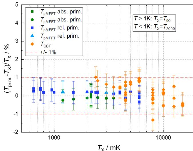
Figure 5: Comparison of pMFFT and CBT in the range of ITS-90 and crucially demonstrating smooth transition in the overlap region between ITS-90 and PLTS-2000 (0.65 K to 1 K)
