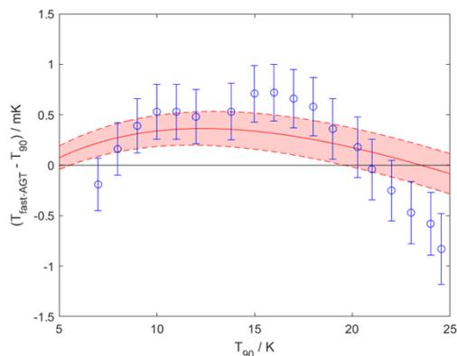
Figure 6: Measurements of  $T - T_{90}$  for fast-AGT. The shaded area is the current best estimate of  $T - T_{90}$ . This shows that for most of the temperature range fast-AGT is an excellent and rapid approach to establishing (and hence disseminating thermodynamic temperature)
