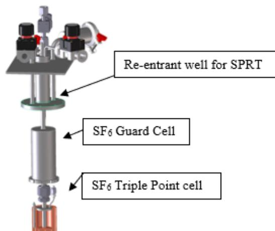
Figure 9: Cross Section of SF<sub>6</sub> calorimeter of LNE CNAM. The whole arrangement is established in a vacuum can and then immersed in an ethanol bath at around -50 °C for realising the SF<sub>6</sub> triple point
