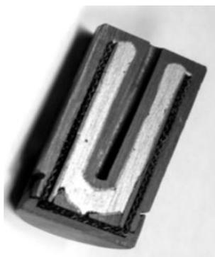
Figure 1: Section through a high temperature fixed point, the shiny metal-carbon ingot surrounds the blackbody tube and is encased within the graphite crucible. The outer diameter is 24 mm.
