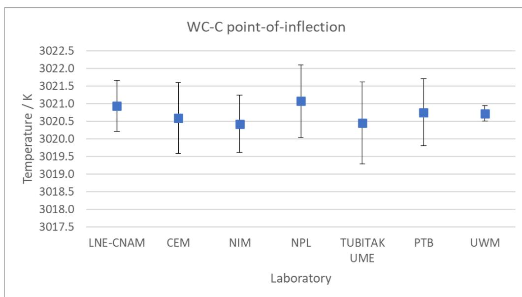
Figure 2: Results of the point of inflection of six independent evaluations (by six NMIs) of the melt of the WC-C metal carbide-carbon high temperature fixed point.
