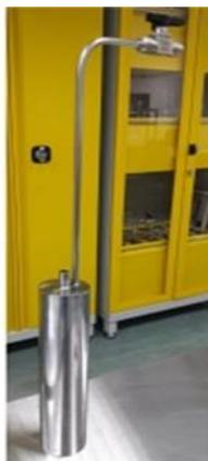
Figure 10: A photograph of a TUBITAK CO<sub>2</sub> triple point cell
