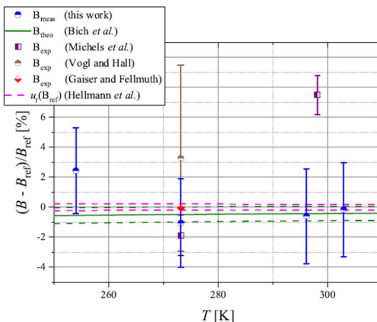
Figure 13: Comparison of experimental data (from PTB) with the measured values of the second density virial coefficient of Ne. Experimental data confirms the calculated values, the latter having the lower uncertainty.
