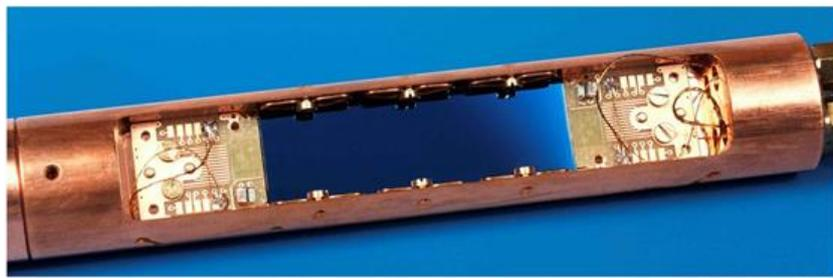
Figure 3: Photograph of a primary Magnetic Field Fluctuation Thermometer (pMFFT)
