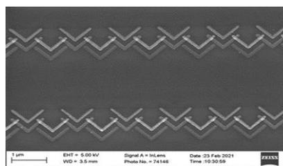
Figure 4: Photograph of a tunnel junction array for a Coulomb Blockade Thermometer (CBT)
