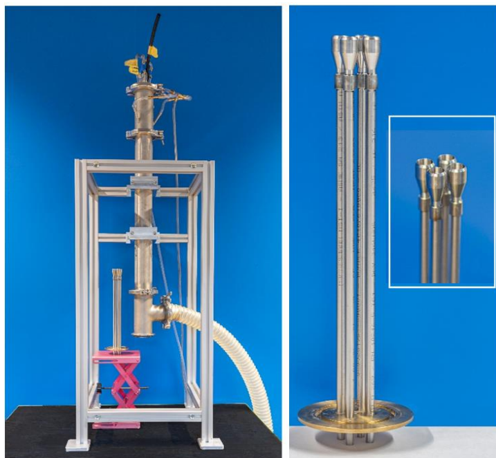
Figure 2. Left panel: Picture of the portable flow tube homogenizer developed and constructed at METAS. Right panel: Isokinetic sampling probes for devices under test (left panel), and close view of the sampling funnel. The sampling probes were designed and constructed at METAS. This figure was first published in (Horender et al., 2022) and is licensed under a Creative Commons Attribution (CC BY) license.
