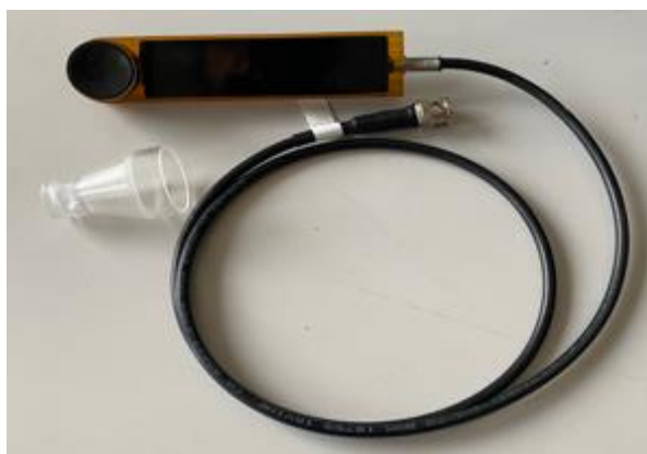
Figure 2 INRIM transducer comprising a SU103 S/N 101, Sonic Concepts transducer with stand-off cone which was filled with deionized, degassed water, and fitted with a Mylar acoustic window for measurements.
