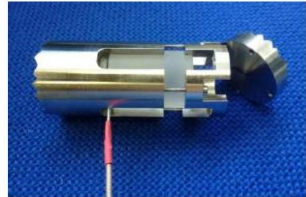
Ultrasonic densimeter prototype
