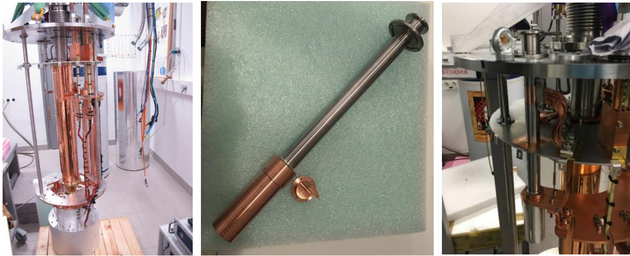
Figure 4.4.3: (left) The cryostat with the vacuum container and heat shield removed. At the bottom can be seen the superconducting magnet coil. (middle) The Josephson standard enclosure consists of a thin-walled stainless steel tube for thermal isolation and a hollow copper end for cooling the Josephson chip. (right) The enclosure mounted in the cryostat with thermal straps to the 50 K plate (aluminium) and the 4 K plate (copper)
