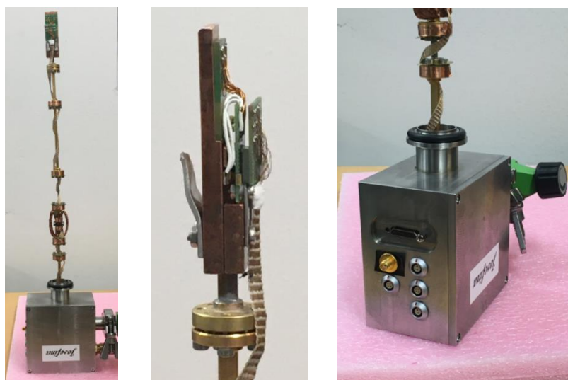
Figure 4.4.4: (left) The Josephson probe is shown upside down. It consists of a connection box at room temperature, a rectangular waveguide with a ribbon cable wrapped around it, and a copper holder for the Josephson chip. (middle) Close-up of the Josephson chip holder provided by PTB. It is made from copper and the Josephson chip (not visible) is firmly glued to the copper for optimum cooling. (right) The room temperature connection box is vacuum
