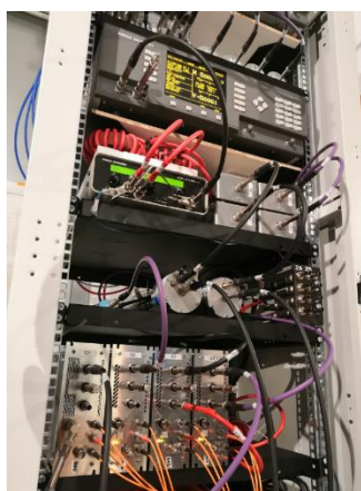
Figure 4.2.3. Left: Digi-Bridge for linking capacitance to the resistance unit. Right: High-frequency bridge with implemented new auxiliary decades and a DDS generator
