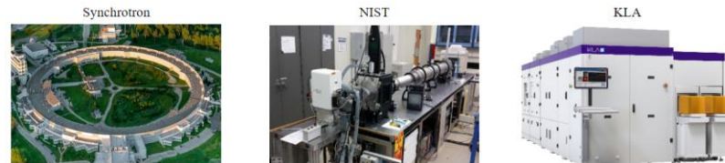
FIGURE 1. CD-SAXS metrology has evolved from synchrotron-based measurements [3] (left) to the pioneering NIST prototype system [4] (middle) to KLA's x-ray metrology system (right), which is a highly sensitive, production-capable metrology system for semiconductor manufacturers.
