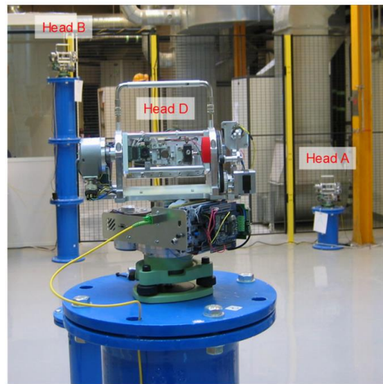
Figure 7 - photograph showing three of the four CNAM measuring heads as part of a multilateration network.
