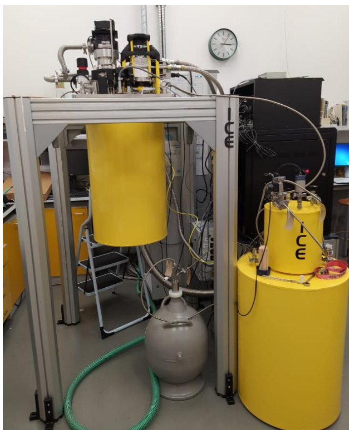
Fig. 14: Photograph of the 300 mK system established for parametric amplifier metrology, the cryostat and cooling system was supplied by the ICE Oxford company in the UK.
