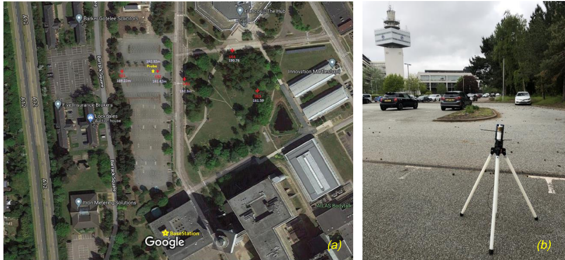
Figure 4 Photograph of the experimental setup for the commercial 5G BS measurement campaign in outdoor environment: (a) map showing the 5G BS and mobile UE locations; (b) setup of mobile UE facing 5G BS.
