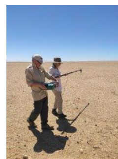
Figure 9: NPL staff measuring surface reflectance of Gobabeb test site.
