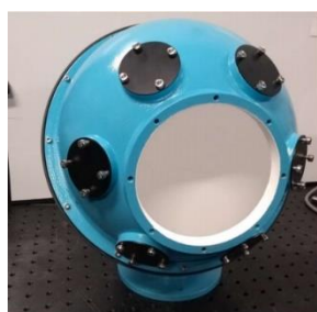
Figure Error! No text of specified style in document.28: Integrating sphere (left) and schematic (right) of the calibration
