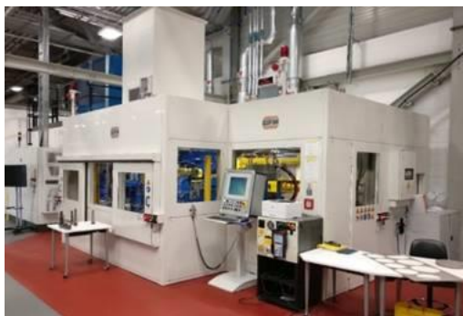
Figure 4.5.8: (left) The radial forge housed at STRATH, UK. (right) Part before (preform) and after forging.
