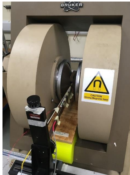
Figure 4.4.8. The three probes – phosphor, thermocouple and resistance – mounted between the poles of the magnet.
