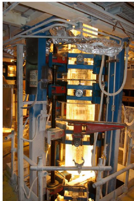
Figure 4.2.3. Quartz glass furnace. The thermocouples are mounted in the die towards the top of the furnace.
