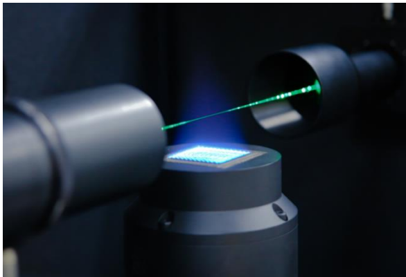
Figure 4.3.1. Left: Portable standard flame being interrogated by the NPL laser Rayleigh scattering apparatus. Right: The gas metering and burner control system.
