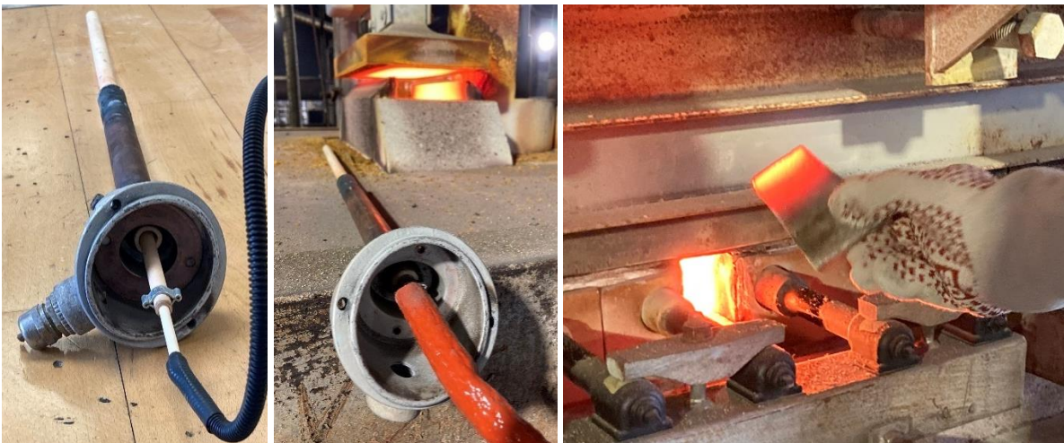
Figure 4.2.7: Left: the thermocouples are installed in ceramic protection tubes. Centre: the thermocouples are preheated on top of the furnace prior to installation to minimize the thermal stress upon installation. Right: access to the floating glass is provided by removing one of the bricks of the furnace.
