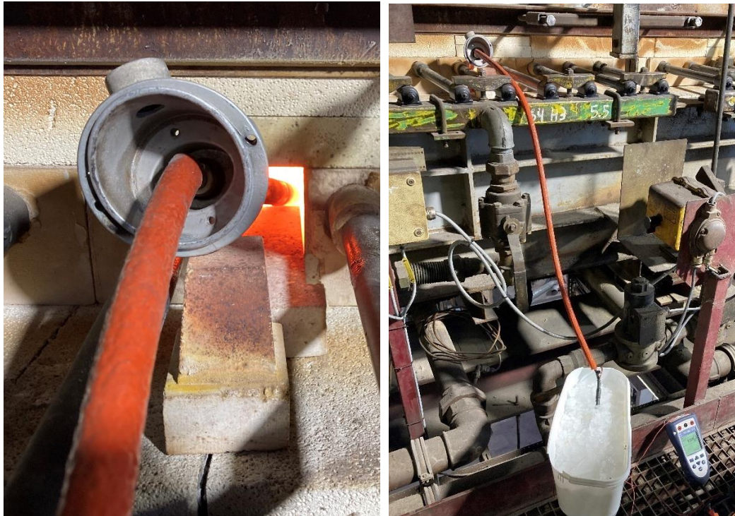
Figure 4.2.8: (left) sensor as installed in the floating glass at approximately 1300 °C, (right) the sensor installation in the glass is seen at the top of the picture and here the cold junction can also be seen.
