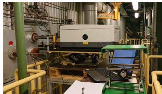
Figure 4.3.5. Top: Filborna WeT waste incineration plant. Bottom: Parallel fast IR emission measurements with IR spectrometer and CEDIP IR camera (left panel: left boiler side) and FTIR spectrometer with sweeping probe (right panel: right boiler side). Both systems are viewing the same axis.
