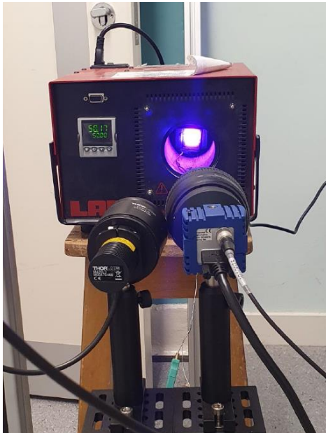
Figure 4.1.5. Top: Experimental layout for phosphor calibration. Bottom left: Experimental apparatus for on-line phosphor thermometry, in the process of being calibrated. Bottom right: Sample output from the on-line thermometry system.
