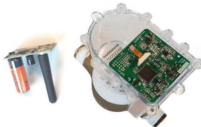
Figure 8 Hardware platform developed for leakage detection based on a low voltage CMOS image sensor, a general-purpose ARM®Cortex®-M4 and a communication part consisting of a RF receiver and a RF front-end module; The electronic device is battery powered with up to 2 low discharge lithium batteries.
