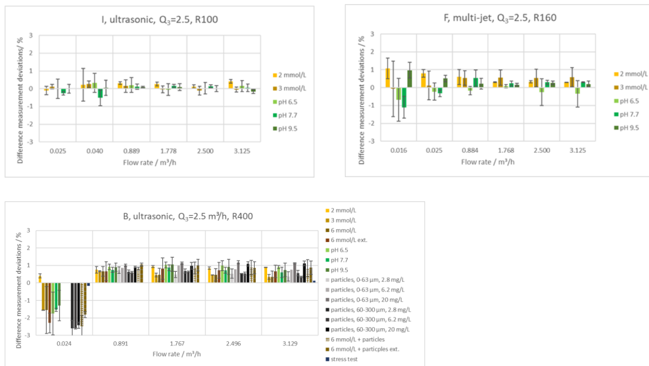
Figure 6 Difference between the measurement deviations obtained at the end of a water quality experiment and the ones for the base measurement. Where standard deviations are included, the average of the results of several water meters is shown. Note the partially different scaling.
