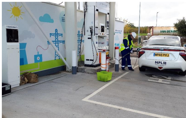
Figure 3: Testing a commercial hydrogen sampling device
