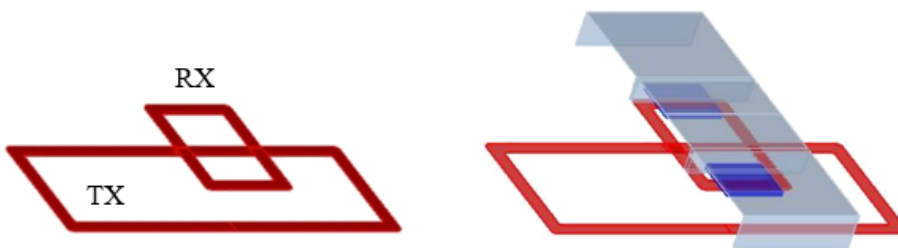
Fig. 7 - WPTS-1: the coil pair, and the complete pad, with aluminum (grey) and ferrite (blue)
