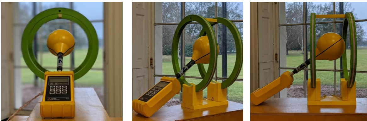
Fig. 18 – The new Helmholtz coil with Narda ELT-400 magnetic field instrument with 100 cm 2 external probe.
