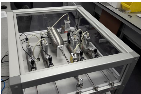
Figure 7 Dynamic mixing facility based on mass flow controllers and a mixing chamber which can be used to generate various biogas compositions (a.o. \text{CH}_4 , \text{CO}_2 , \text{N}_2 ). This facility can be connected to the outlet of the permeation system.
