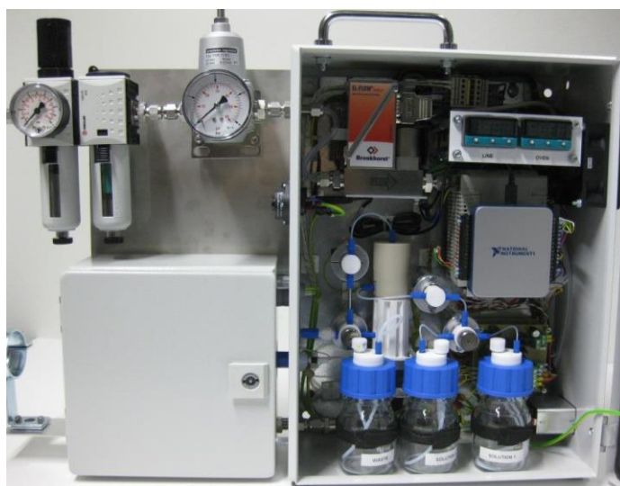
Figure 8 Dynamic generator calibration unit is portable and field deployable.
