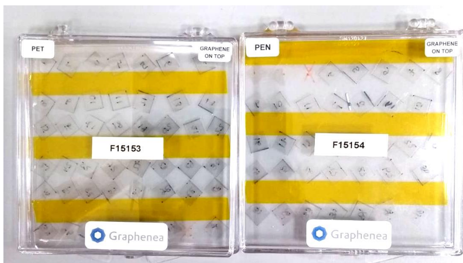
Graphenea synthesized 10 \times 10 \text{ mm}^2 graphene samples on PEN and PET substrates.
