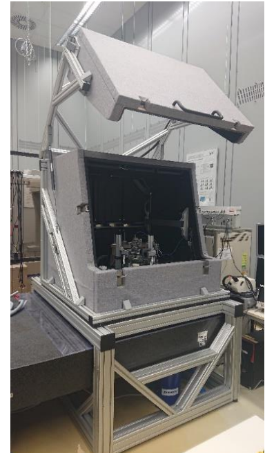
Figure 7. NMM-1 new positioned on heavy granite table standing on pendulum isolators and with new cover for acoustic shielding and isolation.
