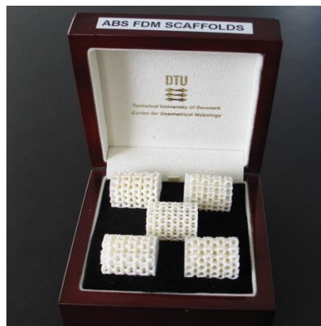
Fig. 1. Parts with defects: 1 without defects, 1 with filled cells, 1 with thicker struts, 1 with thinner struts, 1 with missing struts.
