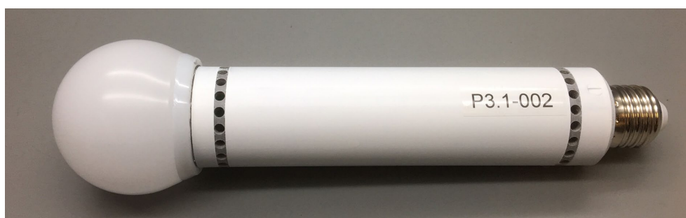
Figure 11. Mains operated led-based lamp for luminous flux.
