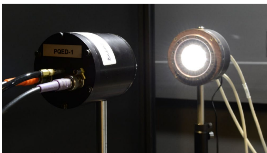
Figure 18. Predictable Quantum Efficient Detector (PQED) measuring a LED-based intensity source.
