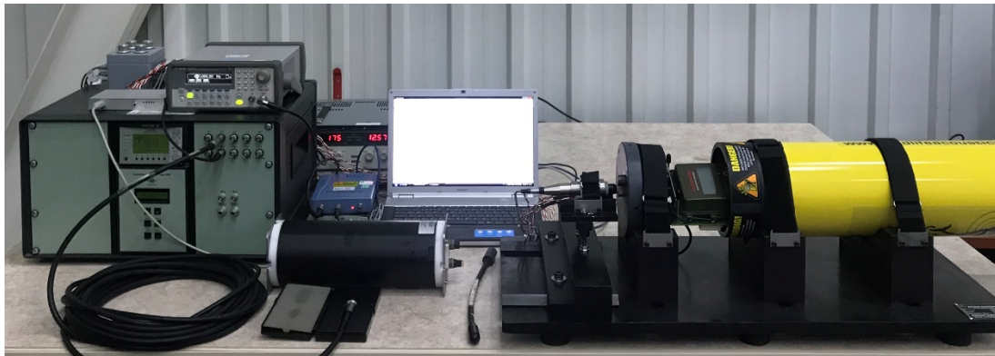
Figure 2: Measurement setup for the calibration of hydrophone and noise recorder
