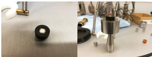
Figure 2.1: Proposed configuration of the reference microphone that minimizes the additional volume on the ear simulator. To the left the WS3 microphone mounted in a quasi-flush adapter; to the right, the microphone mounted on an earlier prototype of the ear simulator.
