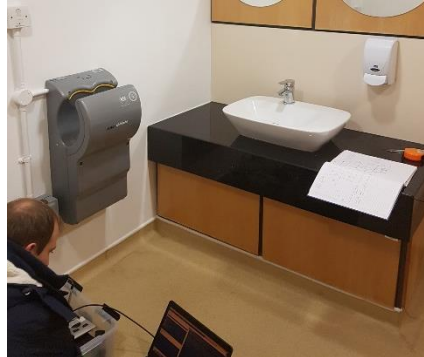
Figure 3.2: Measuring high-frequency sound emitted by a hand dryer.
