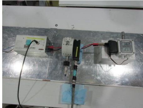
Fig. 13. Conducted immunity test setups of the electronic thermometer with CDN.
