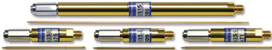
Fig. 1. Air-dielectric lines used as reference standards for S-parameter traceability.
