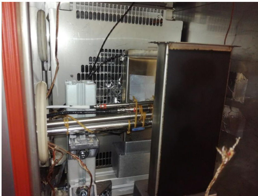
Figure 12. Set-up for studying the effect of direct thermal irradiation on the humidity sensors
