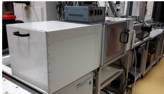
Figure 5. Cover that prevents unwanted condensation at dew-points up to +90 °C
