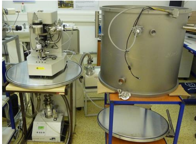
Figure 4.2.1.5: Hermetic chamber capable to contain both an FPG and a DUT and allowing pressure control.
