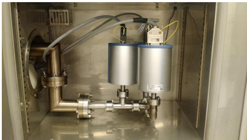
Figure 4.1.4.1: Three INFICON LI CDGs inside a Thermotron 2800 for temperature control.
