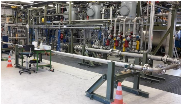
(b) Overall setup at DNV-GL with 10m straight section
