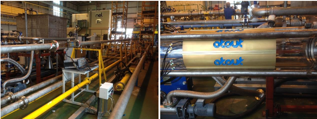
Figure 4.4. ECT sensor mounted on NEL national standard multiphase flow facility, East Kilbride. Close-up view of ECT sensor showing slim-line clamp-on design fitting under tie-rods around existing 140mm diameter sight-tube.
