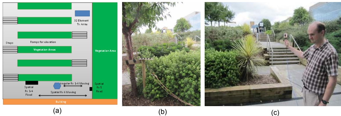
Figure 8 (a) Plan of the outdoor Massive MIMO measurement area and photographs of the measurement environment showing the 32 element transmit array – (b) for Rx1 to Rx4 at a fixed position and (c) for moving Rx 6.
