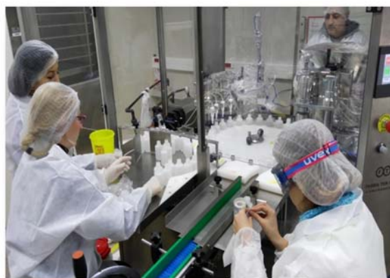
Figure 2: Bottling and capping of the candidate ground water CRM
