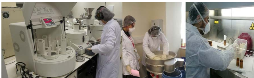
Figure 8. Milling, sieving and filling of soil CRM candidate
