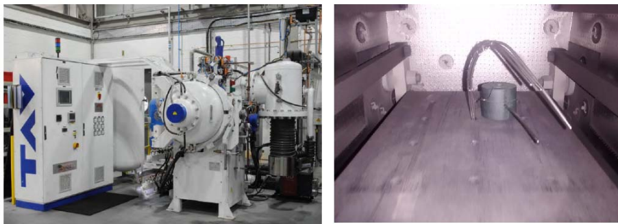
Figure 4.2.7: The industrial vacuum furnace at AFRC (left) and the thermocouples installed inside the furnace (right).
