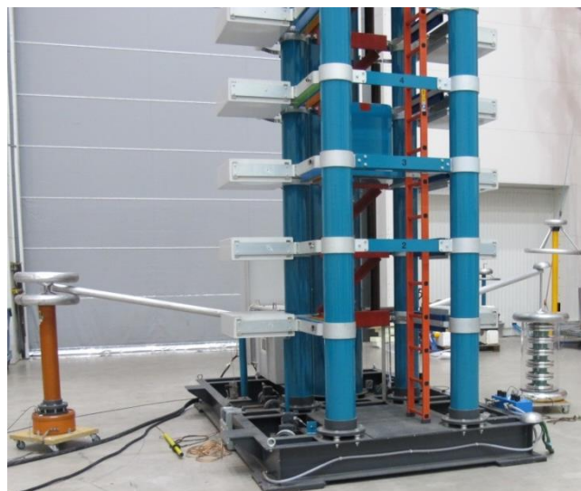
Figure 10: Calibration of the charging voltage measurement of impulse generator. Base of multistage impulse voltage generator in the centre, with the two calibration dividers connected by aluminium tubes on both sides.
