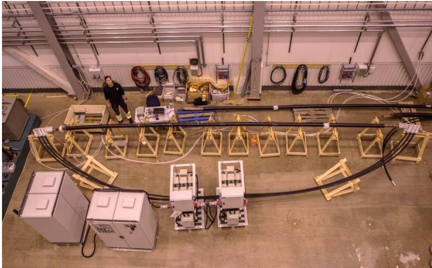
Figure 45. Measurement with AC current in the calorimetric measuring system.
