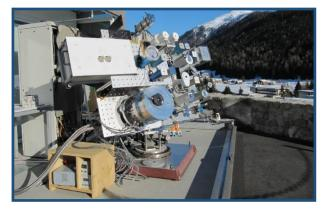
This project has upgraded CSAR, developed in-part during the previous project ENV04 MetEOC. This upgrade allows CSAR to perform continuous sequences of fully automated solar irradiance measurements, incorporate improved cavity absorbance to reach near 100 %, reduce the uncertainty of window transmittance measurement and reduce residual noise to allow measurements at close to 0.01 % uncertainty level. This work has enabled CSAR to be a prime candidate to replace the WRR with a robust SI standard.
