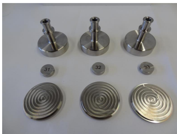
Figure 1: Examples of metal diffusion cells based upon steel In order to cover the range 5 ng Hg/m 3 - 60 µg Hg/m 3 , several types of diffusion cell were made:
