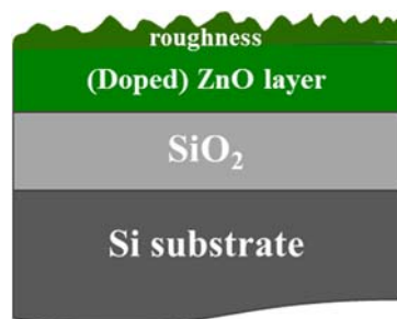
Figure 12: Schematic of the investigated TCO layers produced on thermally oxidised Si substrates
