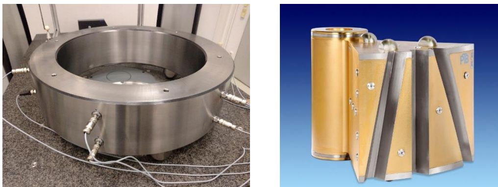
Figure 23: a. Ring measurement standard (left); b. large involute gear measurement standard (right)
