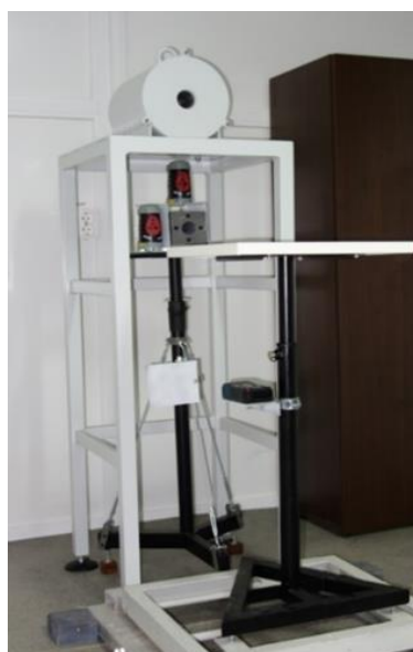
Figure 29: IFIN-HH's low dose rate underground calibration facility.
