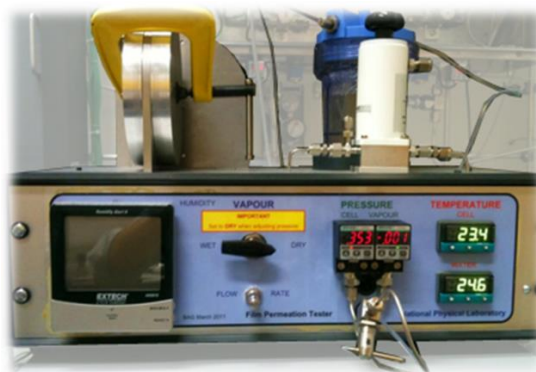
Figure 1 NPL facility for disseminating traceability to industry for measurements of WVTR
