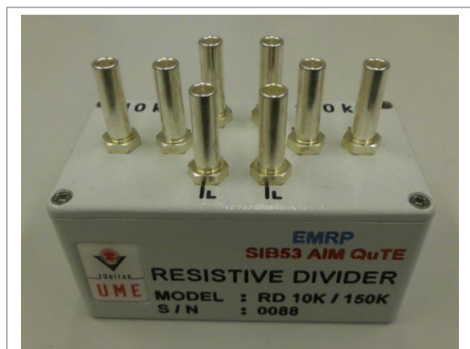
Figure 11 One of the six ratio standards built by TUBITAK.
