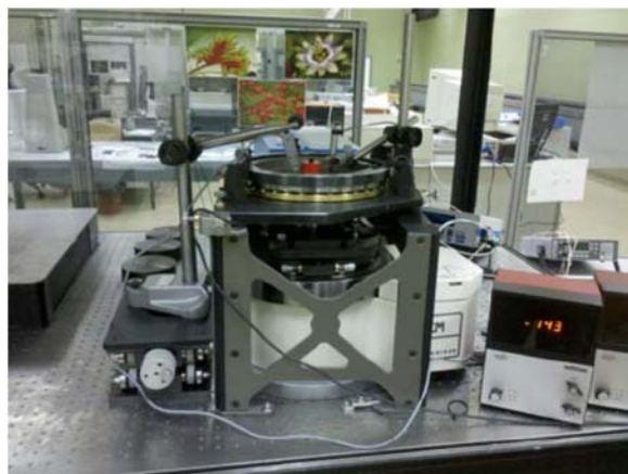
Figure 22. Photos of new tool developed by IK4-TEKNIKER and FAGOR for measuring encoders on the CEM Rotary table
