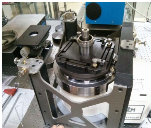
Figure 22. Photos of new tool developed by IK4-TEKNIKER and FAGOR for measuring encoders on the CEM Rotary table
