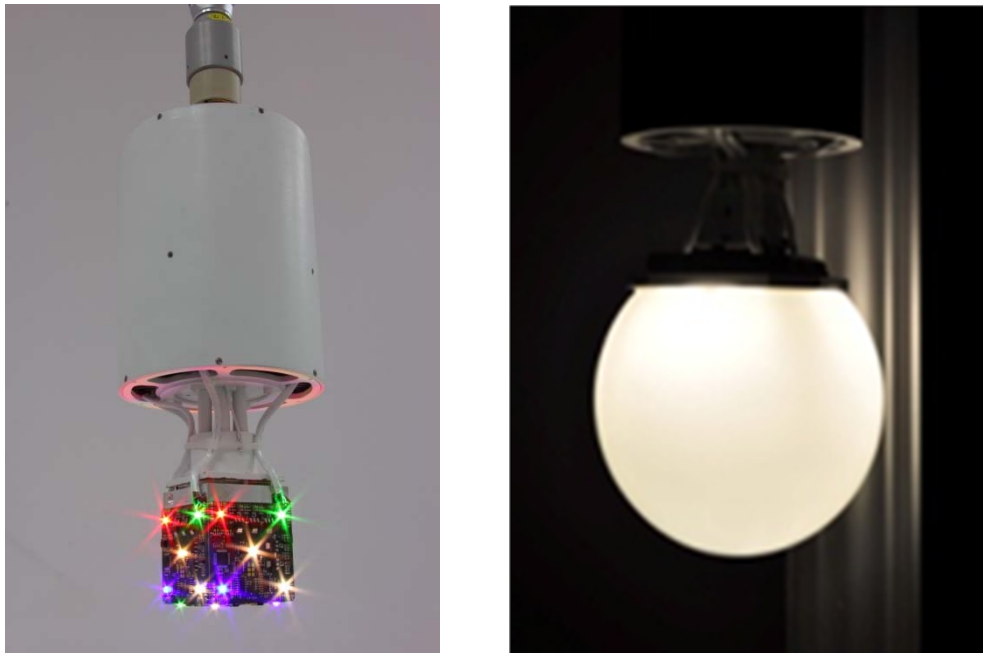
Figure 1. MTS without additional accessories (left) and with diffusing globe accessory (right).
