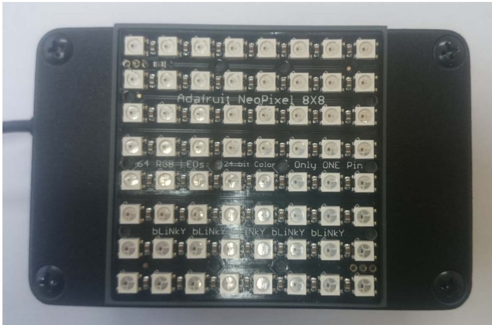
Figure 6. Picture of the LED mosaic to be used as test standard for ILMs.
