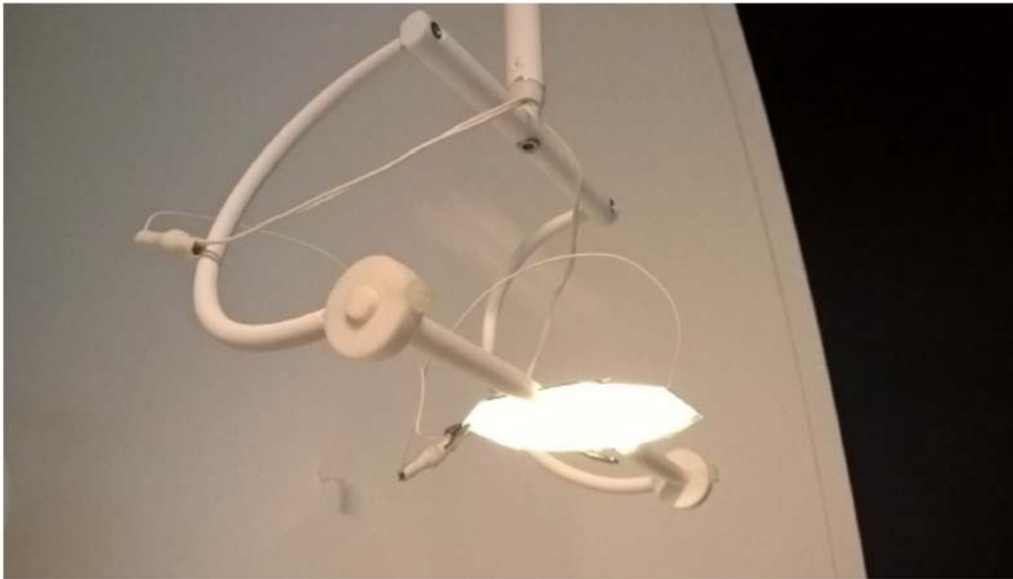
Figure 15. OLED attached to the OLED holder and pointing towards the bottom of the sphere in the integrating sphere measurements.
